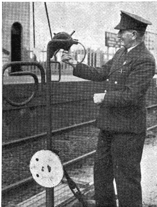
Leading Porter Bill Baldock adjusts the automatic staff exchange apparatus.
